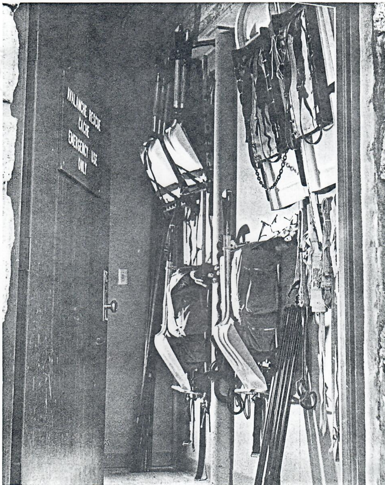
Figure 21.—U.S. Forest Service avalanche rescue cache, Alta, Utah. Cache includes probe poles, shovels, first aid set, and rescue sled.
