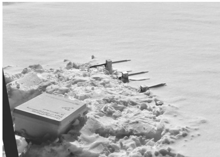
Fig. 2. Photograph showing three vertically oriented pairs of thermistors that were placed in wet snow before dry snow fell. Only the top thermistor of each pair is visible above the dry snow. The thermistors are connected to a datalogger in the white box that reads each temperature every two minutes and records the average temperature of each thermistor every hour.
