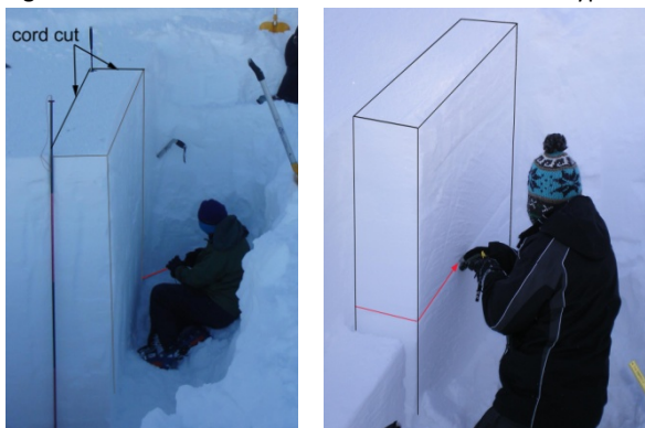
Fig. 2: Isolating a PST column (left) and saw-cutting upslope along the weak layer with the blunt edge (right).
