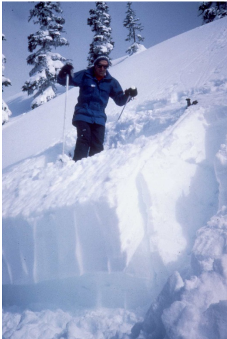
Peter Schaefer demonstrates a Swiss rutschblock test during one of his early visits. Bruce Jamieson photo.
