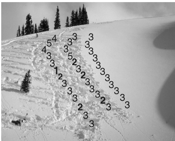
An array of rutschblock tests on a weak layer of surface hoar from 1991. Mark Shubin and Bruce made the third row of tests after the photo was taken. Note that a single test in the top left part of the array gives a misleading indication about local stability. Bruce Jamieson photo.
