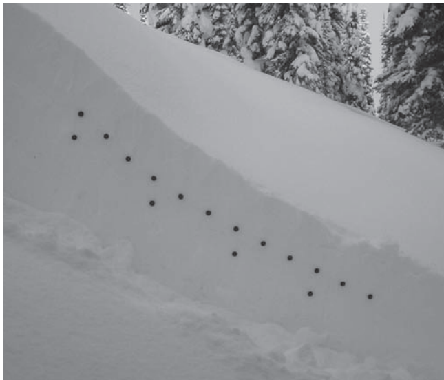
This photo was taken before one of Alec van Herwijnen’s fracture speed tests. The markers are rubber corks, and the weak layer is in between the two rows. He filmed the propagating fractures with a high-speed video camera, capable of capturing 250 frames per second.
