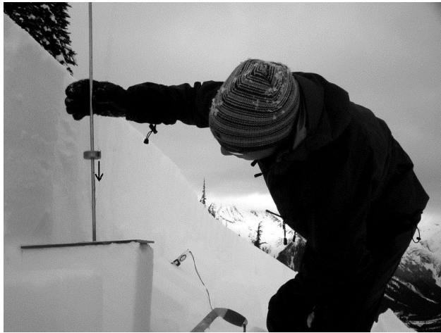
Figure 12. Cam Campbell demonstrates a drop hammer tester, consisting of a rigid 30 cm x 30 cm plate with a perpendicular guide rod. A brass weight (hammer) is dropped along the guide rod from 5 cm, 10 cm, etc. until the weak layer fractures across the column. From the weight of the hammer, 300 g in this photo, and the drop height, the energy delivered to the top of the snow column can be calculated. For these deep tests, the snow in the column is consolidated and no crushing is observed. Since much of the energy from the tester probably arrives at the weak layer, the energy required to fracture the weak layer can be calculated.
