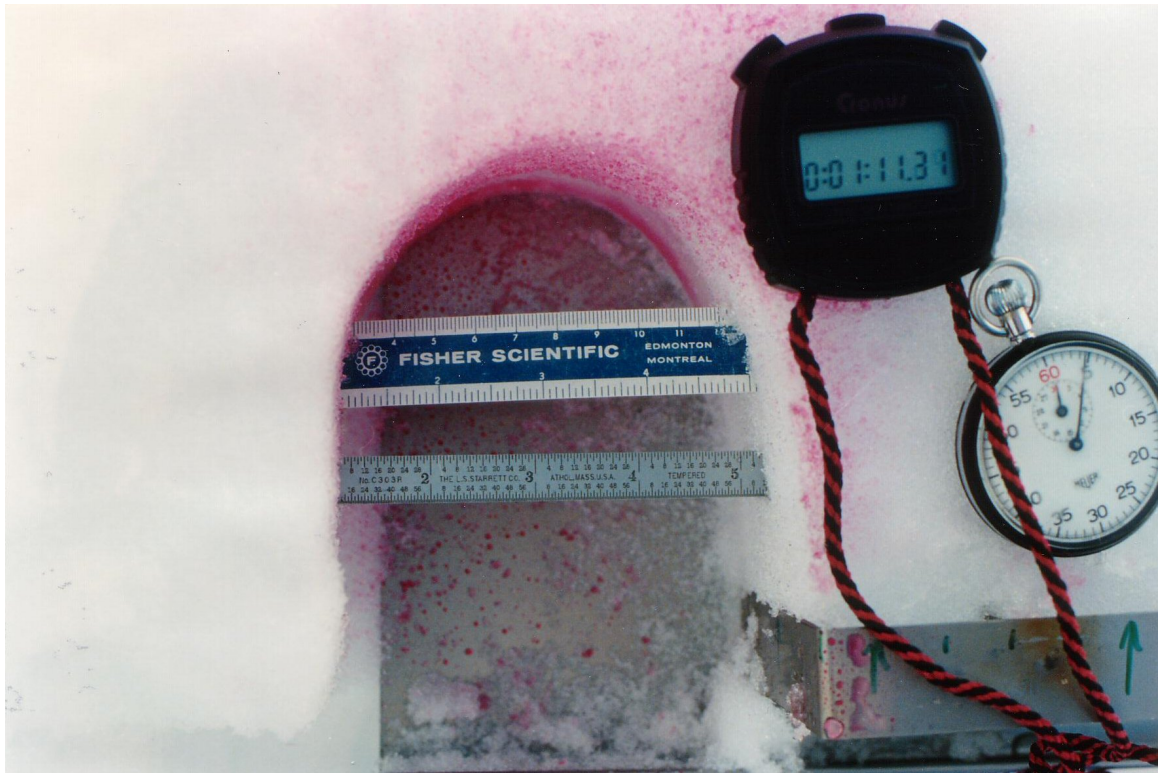
Figure 5.6: Measurement of Notch Deformation During Loading
