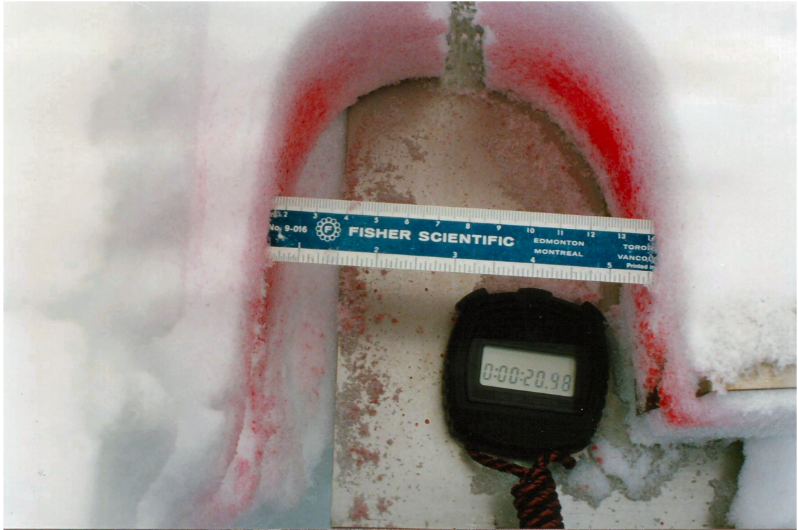
Figure 5.7: Displacement of Snow Block and Fracture Surfaces
