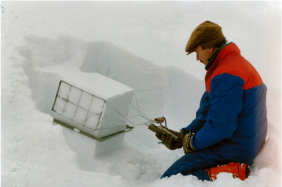
Figure 3.2: Tensile Test on an 18^\circ Slope
