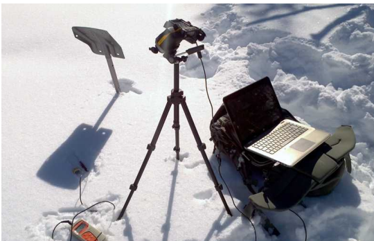
Figure 6. Experiment in 2014 to compare the readings from two contact thermometers in the shade of the shovel and an IR thermometer (not shown).
