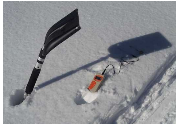
Figure 5a. Shading of the snow surface by a shovel blade on a clear day. The temperature in the shade is being measured with the two contact thermometers.
