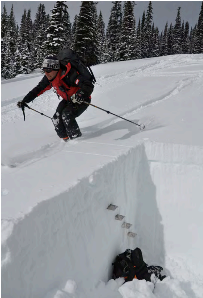
Figure 1: Mike Wheater loading the snow surface above the sensors. The sensors are mounted to long aluminum sheets which are inserted into the side of the profile. The data logger is in the black bag.
